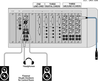
11. In the CONTROL ROOM section on the right side of the console, turn the level control all the way down (counterclockwise), and select L-R for the source and NEAR (Speaker Out A) for the output.
